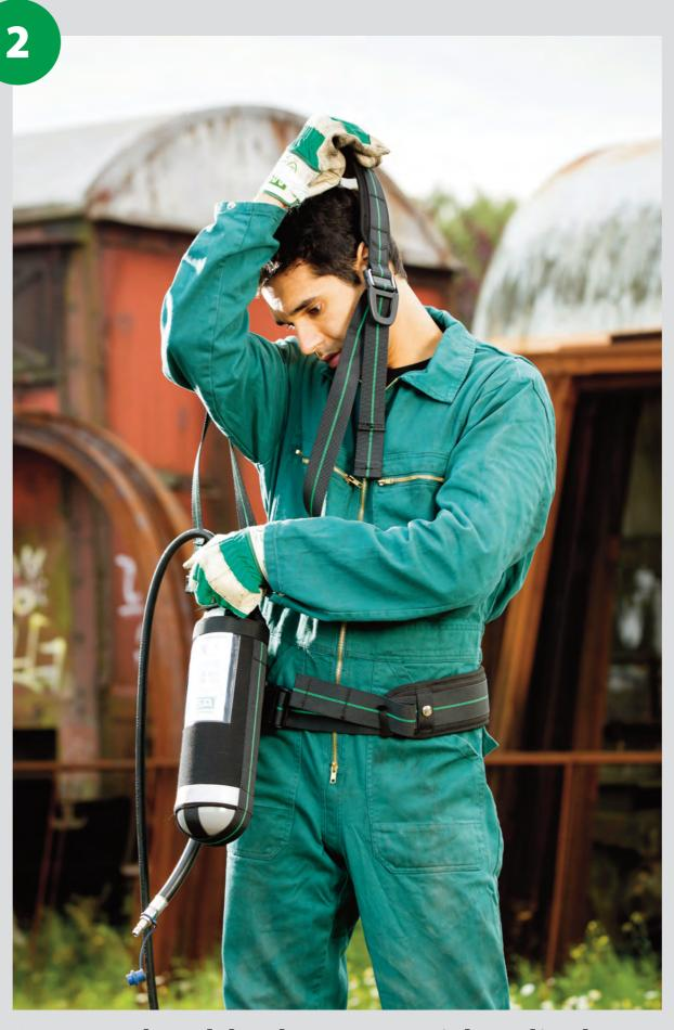
Put on shoulder harness with cylinder demand valve airline assembly.
