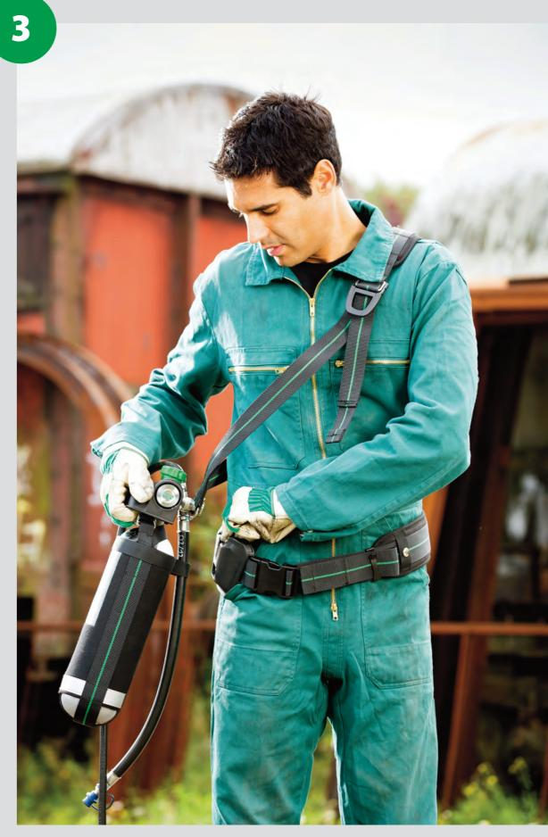
Attach cylinder to holster assembly and adjust shoulder strap.
