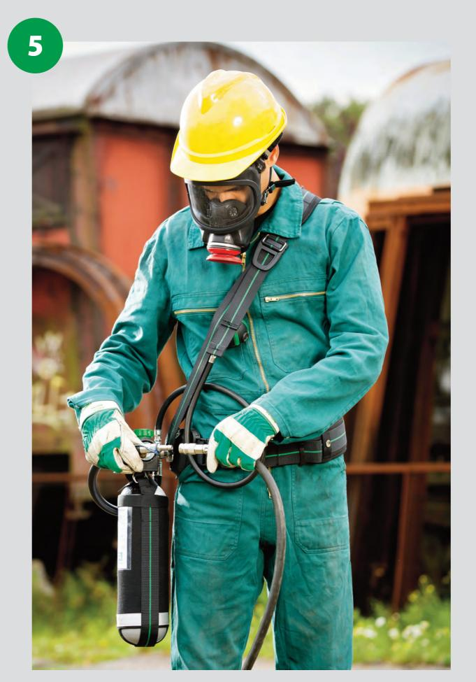
Check gauge to ensure fully pressurized cylinder. Pull on airline hose, remove protection cap and connect pigtail to airline.\*
